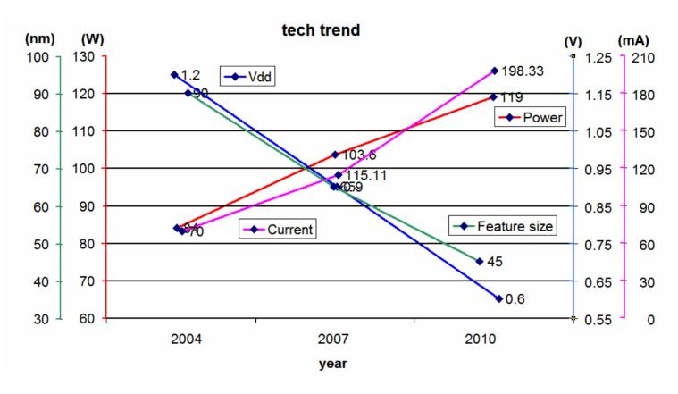
with process size shrinking, system voltages dropping, load currents rising, and clock rates increasing, good PDS design is now crucial to system performance.
