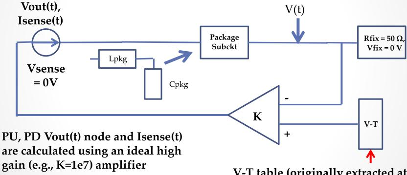
V-T table (originally extracted at the Fixture) is now a PWL driver
