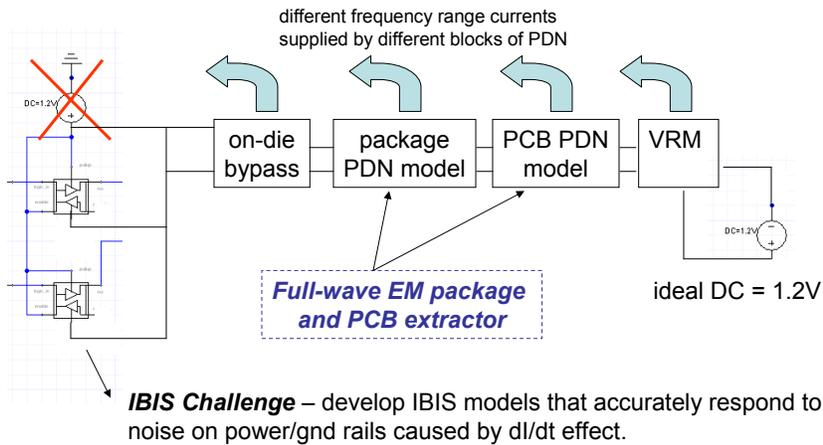
**IBIS Challenge** – develop IBIS models that accurately respond to noise on power/gnd rails caused by  $di/dt$  effect.
