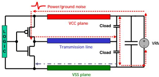
When the output is driven high, the transmission line is connected to the PWR net at the driver. When the output is driven low, the transmission line is connected to the GND net at the driver. This connection forms one end of the sig/gnd or sig/pwr loop.
