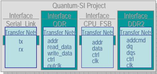
Each interface kit contains net class schematics, timing data & SI models
