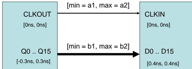
$$\begin{aligned} \text{Setup margin} &= [\text{early clock}] - [\text{late data}] - [\text{setup requirement}] \\ &= [0\text{ns} + a1] - [0.3\text{ns} + b2] - [0.4\text{ns}] \\ &= a1 - b2 - 0.7\text{ns} \end{aligned}$$
