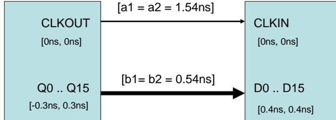
$$\begin{aligned} \text{Setup margin} &= a1 - b2 - 0.7\text{ns} \\ &= 1.54\text{ns} - 0.54\text{ns} - 0.7\text{ns} \\ &= 0.3\text{ ns} \end{aligned}$$
