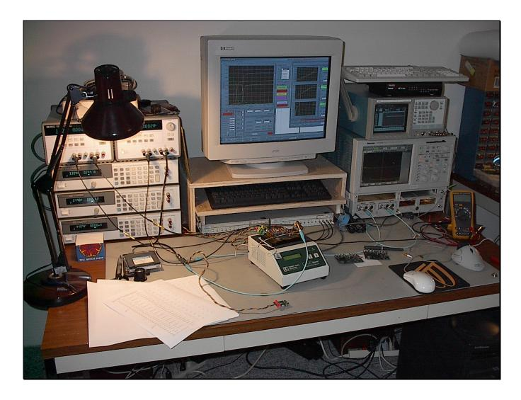
This is one of Teraspeed's test setups. There are 5 power supplies, one scope with 20 GHz sampling heads and a 24 channel word generator. Also pictured is a hot/cold plate to vary the case temperature from 0 to 100C. There are a lot of other tools required such as probes, attenuators, etc.
