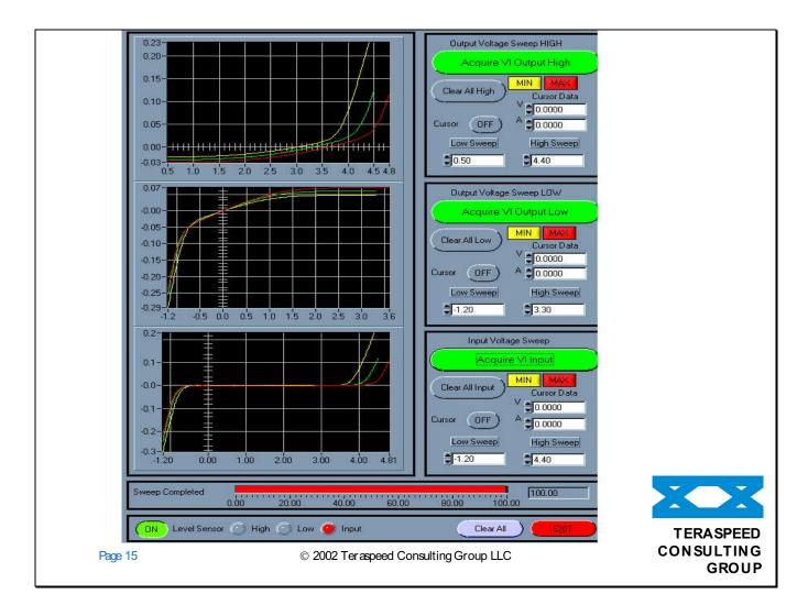
These are the IV characteristics of the same component over process, temperature and voltage. The upper window shows the pull up characteristics, the middle the pulldown and the lower the input.
