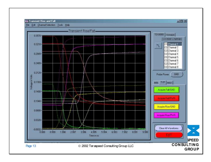
Here is a complete set of VT curves for a part measured over process, temperature and voltage. The upper set of waveforms are with the 50 Ohm termination tied to Vcc and the lower set for the output terminated to ground. It is easy to see the change in prop delay in the component from the max to typ to minimum set of conditions.
