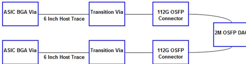
Host board PCB is 26 Layers, total 4mm thickness, M7N level material.
