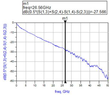
Loopback channel insertion loss
