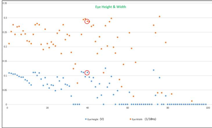
✓ COM recommended EQ parameters produce a good time domain eye diagram
