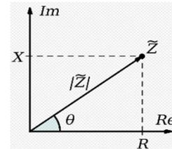
*For a high-speed I/O buffer, the buffer inductance and capacitance are specially designed. It is close to minimum for the reactance  $X$ . So, in this case, the resistance  $R$  is the main factor for impedance matching.*
