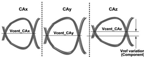
Figure 180 — Across pin  $V_{REF-CA}$  voltage variation
