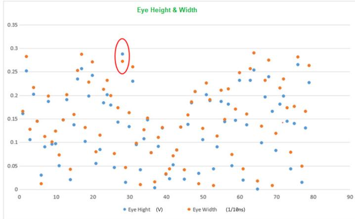
✓ COM recommended EQ parameters produce an acceptable eye opening, but possibly less optimal than the eye opening obtained by time domain simulation
