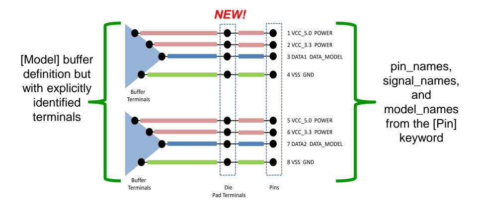
Introduces optional Die pad interface for terminals separate from Buffer and Pin interface terminals
