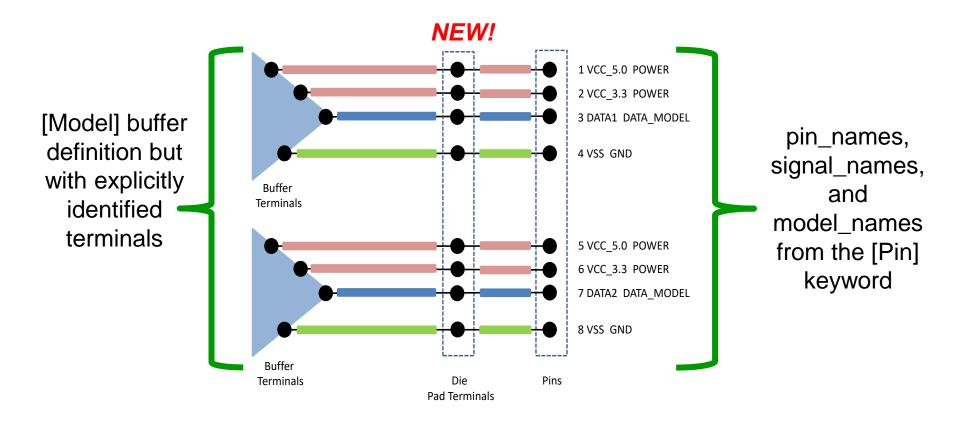
Introduces optional Die pad interface for terminals separate from Buffer and Pin interface terminals
