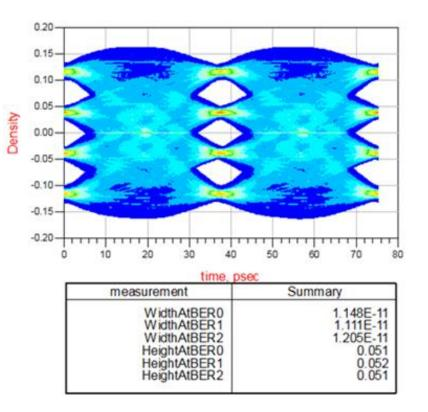
• Simulation results show that the channel including a 11.4 inch trace with one connector can meet the eye height requirement of the CEI-56G-VSR-PAM4 specification at TP1a.
