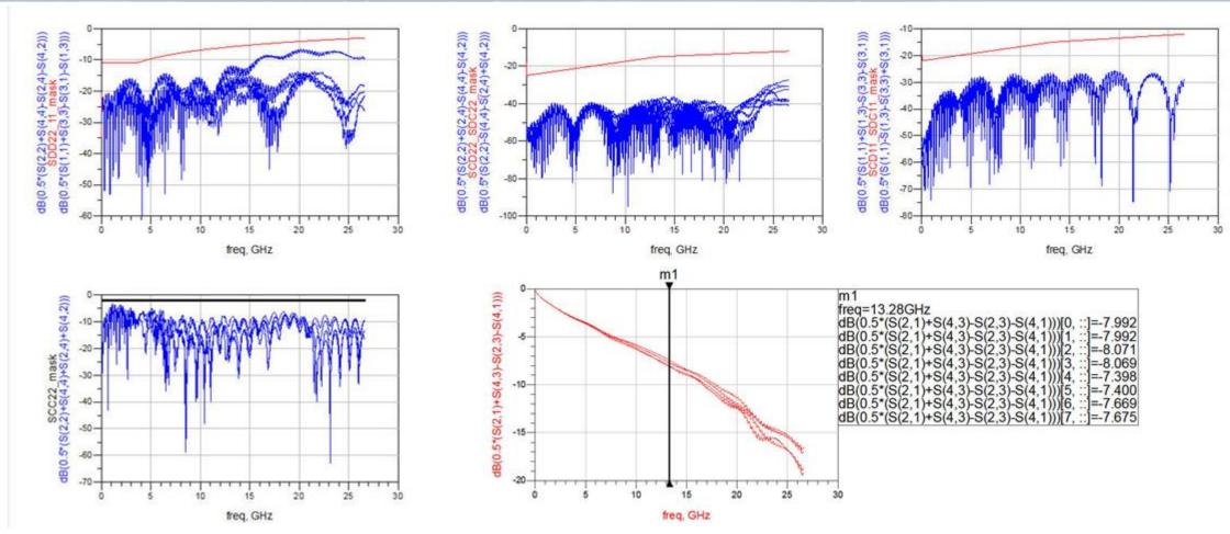
• Simulation results show that the channel including an 11.4 inch trace with one connector can meet the passive requirement of the CEI-56G-VSR-PAM4 specifications.
