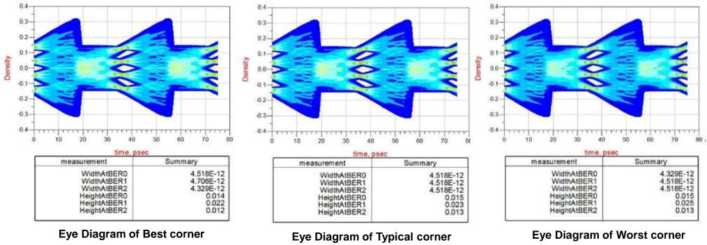
Simulation results show that the channel including two 11.4 inch traces can support the 3m 28AWG QSFP-DD cable for 53.125G rate.
