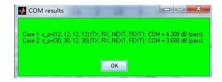
Simulation results show that the channel including two 11.4 inch traces with the 2.5m 28AWG QSFP-DD cable assembly, can meet the IEEE802.3cd/D2.2 Specification COM requirement for 200GBASE-CR4 based on the default package S parameters for both cases.
