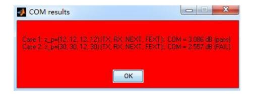
Simulation results show that the channel including two 11.4 inch traces with 3m 28AWG QSFP-DD cable assembly, Case1 can pass and Case2 cannot meet the IEEE802.3cd Specification COM requirement for 200GBASE-CR4 based on the default package S parameters.
