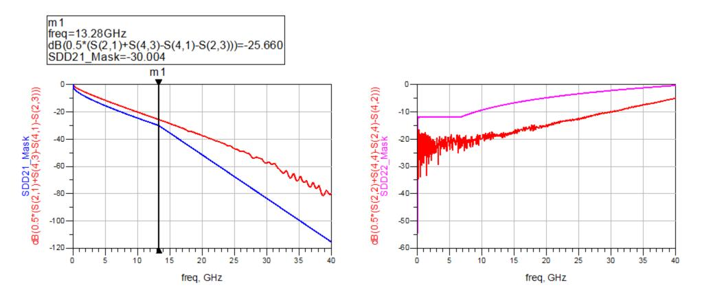
The simulation results are shown above. The channel includes an 11 inch trace on the Switch Card, a 7 inch trace on the I/O Card and one connector. The channel can meet the 200GBASE-KR4 specifications of the passive channel requirements.
