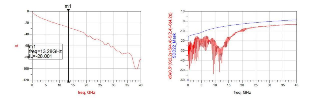
Simulation results show the IL/RL of two 11.4 inch channels with 3m 28AWG cable loop back can meet the 200GBASE-CR4 specification passive requirements.
