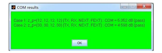
• Simulation results show that the 11 inch trace in Switch Card and 7 inch trace in I/O Card can pass the COM specification with default package model.
