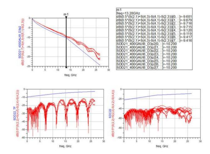
• Simulation results show that the channel, including 11.4 inches of trace, can meet the 400GAUI-8 C2M specification passive requirements.
