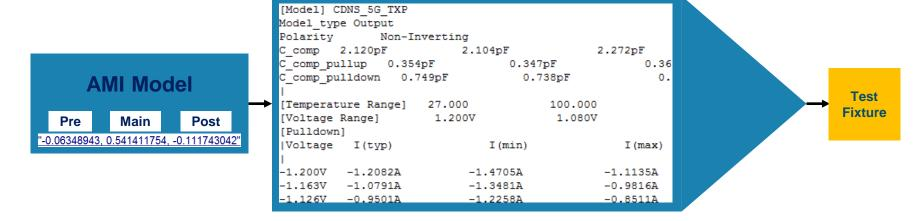
1. Transistor model with EQ on – Circuit Simulation (1,024 bits transmitted) To qualify the **IBIS-AMI** model so generated. 2. IBIS-AMI model – Channel Simulation (1e+16 bits transmitted)
