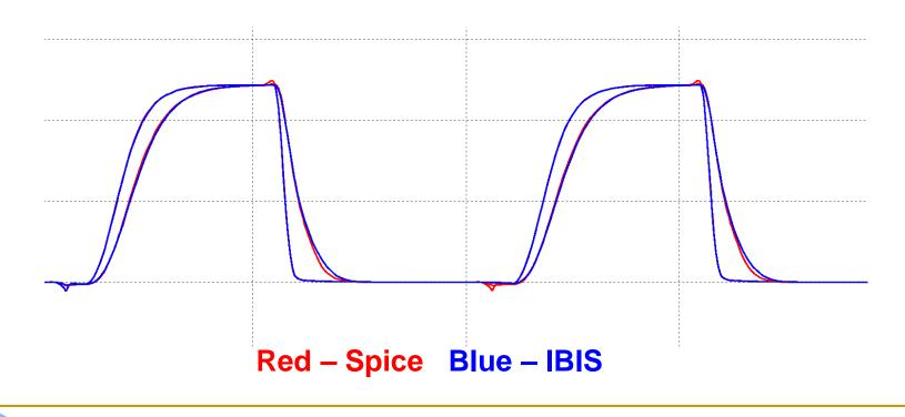
The result from the load with capacitance correlates well with Spice simulations for C\_fixture=15pF IBIS Model
