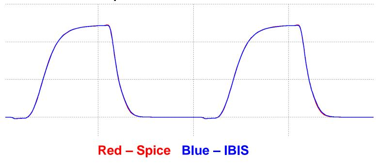
The slight difference in results from the load without capacitance for C\_fixture=15pF IBIS Model
