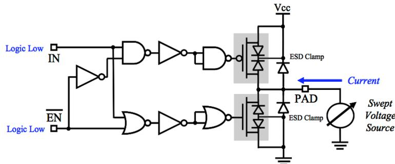
Figure 3.1 – Standard 3-state Buffer (Pull-down I-V Table Extraction Shown)
