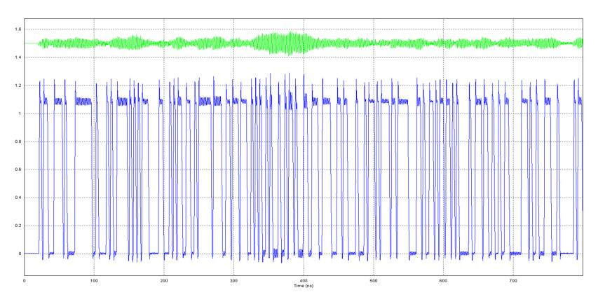
While performing SSO analysis with random bits pattern, lower frequency transition bits may meet the middlefrequency resonance and lead to larger power/ground noise and worse signal quality.
