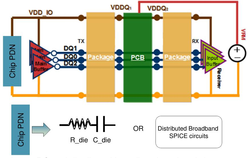
Lump RC and distributed broadband model will be applied for SSO analysis with PRBS patterns
