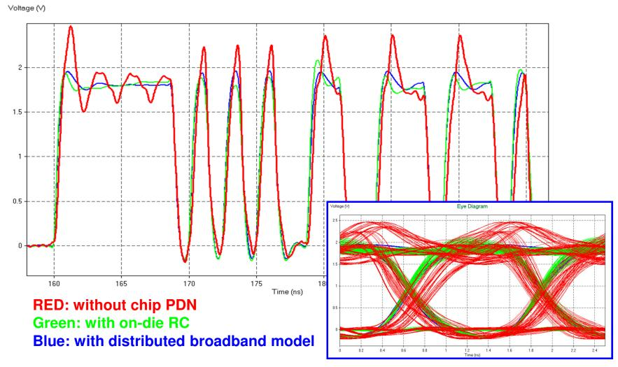
Without Chip PDN model, artificially large power/ground noise impact the signal waveform significantly
