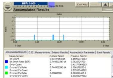
More than 12 hours of the bit error rate test, the emergence of four errors.
