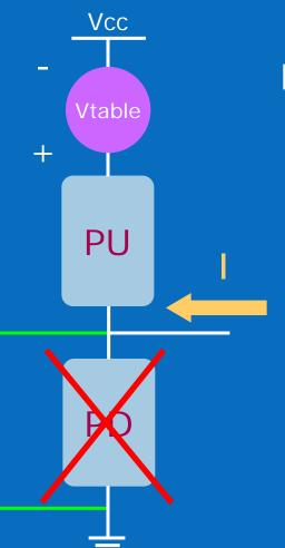
Measure the current as voltage is swept from –Vcc to Vcc (relative to Vcc!)
