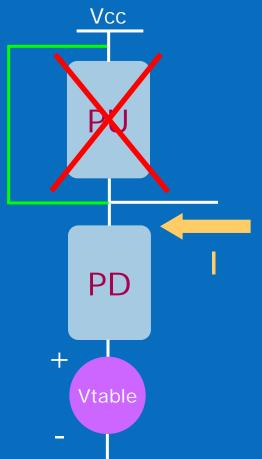
Measure the current as voltage is swept from –Vcc to Vcc
