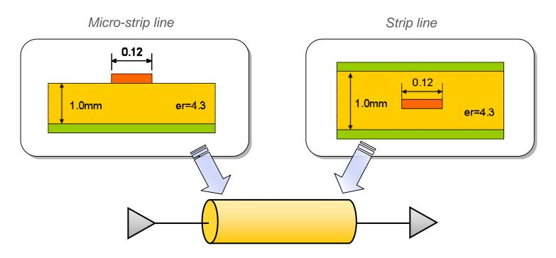
Template of the cross-section models of the transmission line is pre-defined.
