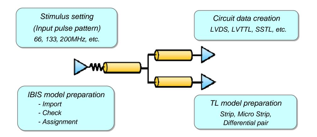
Complicated preparation task can be reduced by providing these initial templates.
