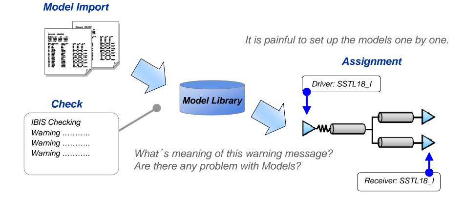
All processes from the model import to the model assignment are implemented in advance.
