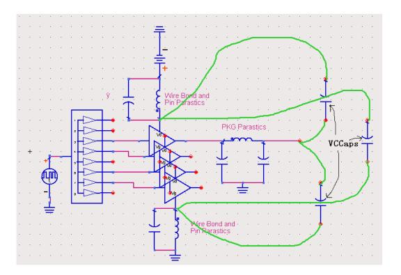
The subcircuit consists of three separate Voltage Controlled Capacitances (VCCAPs) that are placed between the power and ground rails, the output and the power rail and the output and the ground rail
