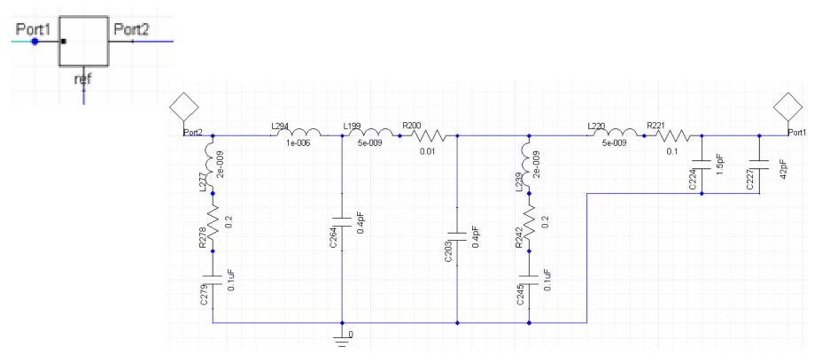
for simplifying, the 2-Port composed of RLGC component is applied
