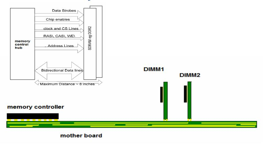
A typical DIMM structure of memory channel
