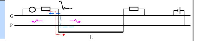
Multiple signals switching with reference plane change
