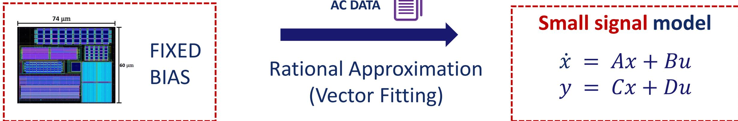
Once the small signal model is available, compute the required  $Y_C$  from a DC analysis. **Equivalent netlist** synthesis is possible
