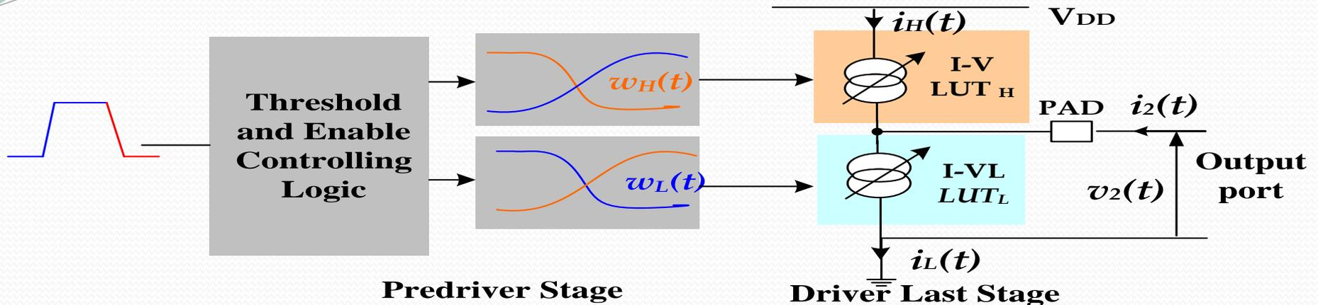
Basic elements of the digital IBIS output buffer behavioral model.
