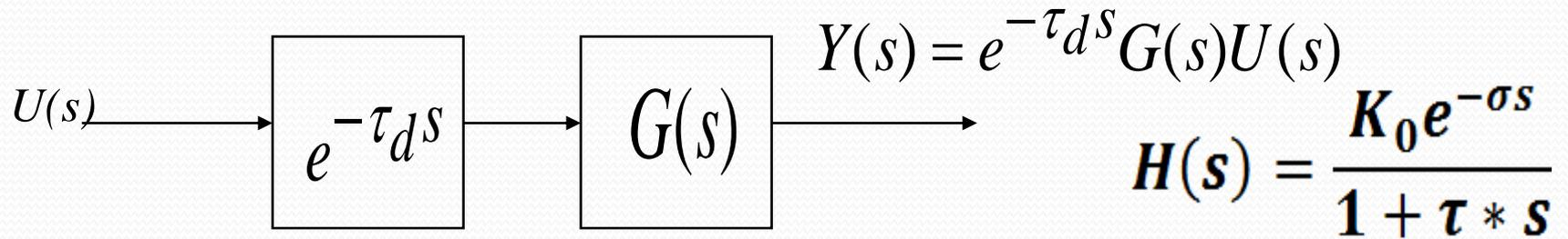
$K_0$  is the dc voltage gain. The  $\sigma$  is dead time between the step excitation and the response. The low pass filter time constant is  $\tau$ .
