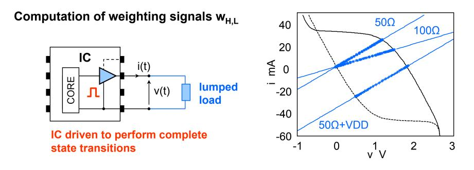
$w_{\rm H,L}$  obtained by linear inversion of model equation
