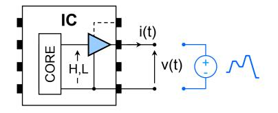
for w<sub>H,L</sub>: transient responses while the port is connected to reference loads and performs state transitions (e.g, 50 Ω resistor)
