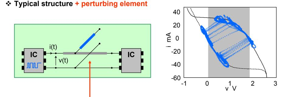
Simplest (passive) **perturbing element**: stub (time delay > 1/3÷1 bit time)
