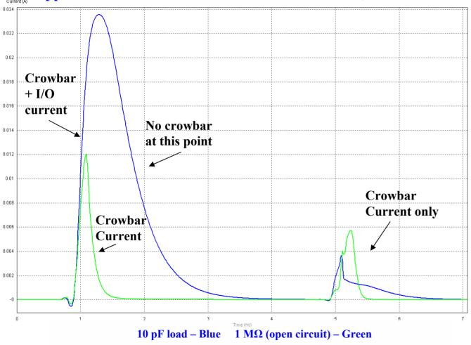
This slide compares the final stage's crowbar current at the high-to-low transition at 5ns. All loads are fully charged to VDDQ before the transition begins, thus the upper device current is the crowbar current.
