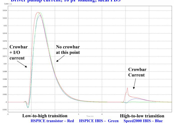
The magnitude of the rising-edge pullup current is dominated by the I/O current that charges the load capacitor. Both IBIS algorithms show good correlation to the SPICE model for the rising edge pullup current.
