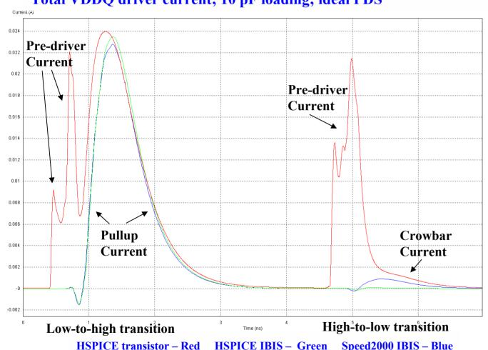
The total VDDO current for the transistor-level model is significantly different from its pullup component. There is a large amount of pre-driver current due to crowbar effects and gate capacitance charging.
