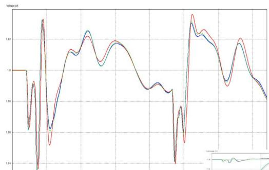
The IBIS simulations now show excellent correlation with the SPICE results over the full simulation. With the addition of the RC circuit, the oscillations occur at the proper frequencies and the SSO magnitude is correct.
