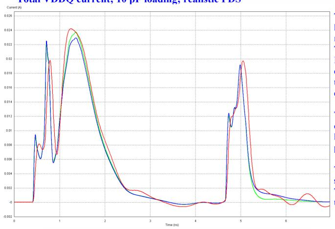
The PWL pre-driver current has a higher dI/dt than the realistic pre-driver current. The difference is because the PWL pre-driver current was extracted with an ideal PDS that facilitated the optimistic dI/dt.
