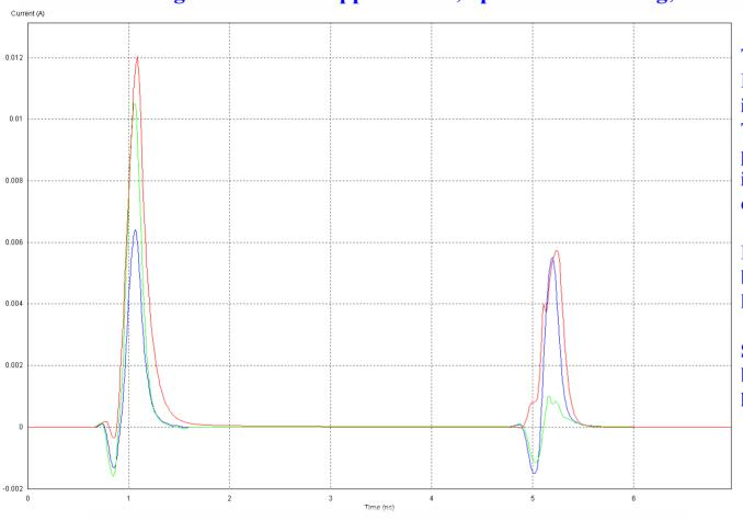
The IBIS algorithms in HSPICE and Speed2000 include the crowbar current. The overlap of the pullup and pulldown current sources is inherent in the model and cannot be excluded.
