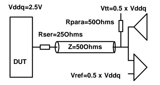
SSTL\_2 Class I symmetrically single parallel terminated output load and series resistor
