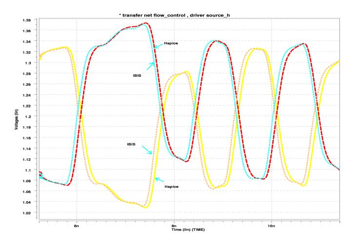
SPI4 interface: 1.25GHz, target pad, VDDQ=2.375
