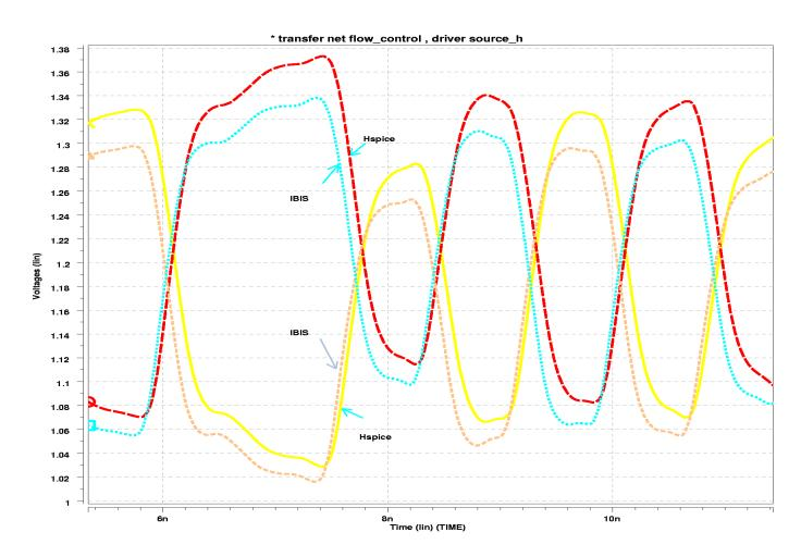
SPI4 interface: 1.25GHz, target pad, VDDQ=2.325, Model generated w/VDDQ=2.375
