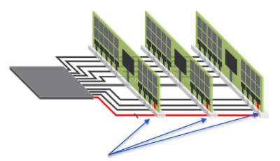
Multi-drop topology of DDR bus causes channel loss, limits speed
