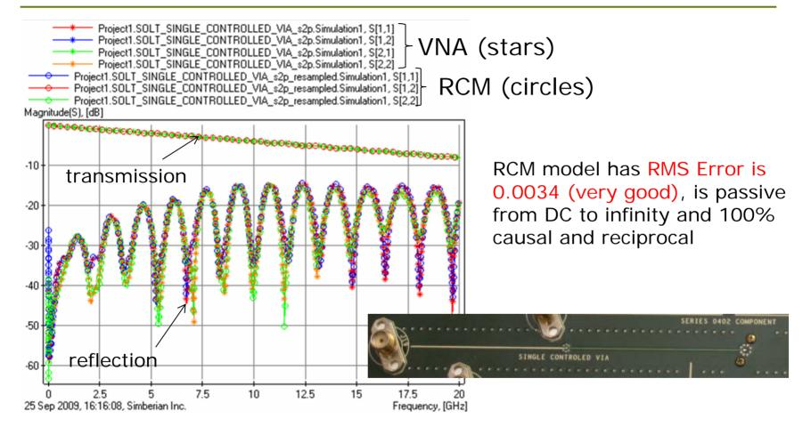
Touchstone model with DC and reduced number of frequency points or BB SPICE model can be produced from RCM
