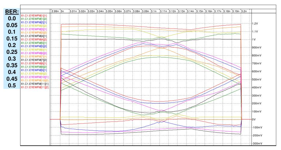
The Rx model has an array parameter (BERvalues) through which the user can request which and how many eye contours should be plotted. Each contour corresponds to a certain BER.
