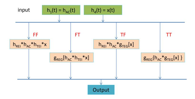
Each branch contains four components of: (1) stimulus; (2) Tx AMI; (3) analog channel; (4) Rx AMI
