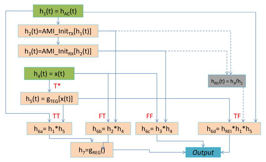
Four possible combinations of Tx GetWave\_Exists and Rx GetWave\_Exists are: FF,FT,TF and TT
