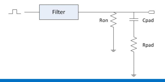
Initial finding: this <u>cannot</u> be modeled without IBIS-ISS, External Circuit, External Model, or some other post-4.0 feature
