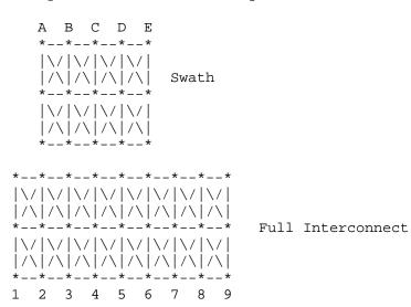
Centering is a way to map the swath matrix pins directly into the corresponding pins of the actual interconnect. For example, the swath above is centered about column 4 of the full sized interconnect. The paths of interest, including those of columns 3 and 5, are also described by swath matrix data that has coupling from both sides. However, because of edge effects, columns 2 and 6 are less accurately approximated by the corresponding swath columns (A & E, respectively).
