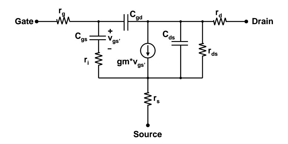
Typically, all capacitances are voltage dependent (function of Vds/Vgs), and rd/rs are not that small
