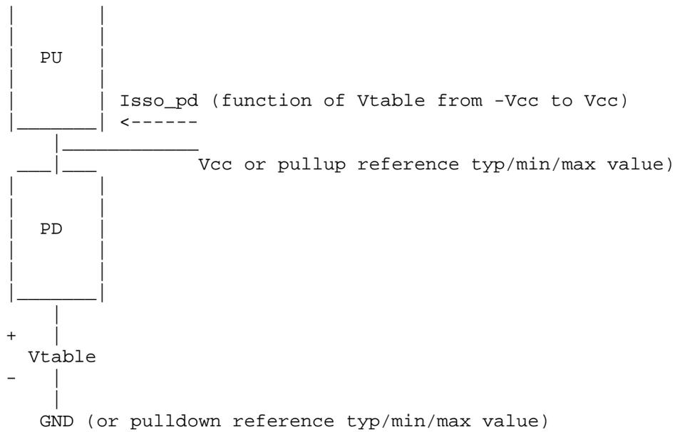
The effective current table for the `Ippo_pu` current is extracted by the following process. The buffer is set to "logic one". A `Vtable` voltage source is inserted between the [Pullup Reference] node and the buffer as shown below. This `Vtable` voltage is swept from -Vcc (typical) to +Vcc (typical) and is relative to the [Pullup Reference] typ/min/max values for the corresponding columns. The output is connected to the Vcc (typical) value as shown below.
