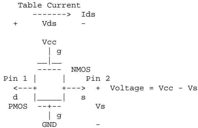
Either of the FETs could be removed (or have zero current contribution). Thus this model covers all four conditions, off, single NMOS, single PMOS and parallel NMOS/PMOS.
