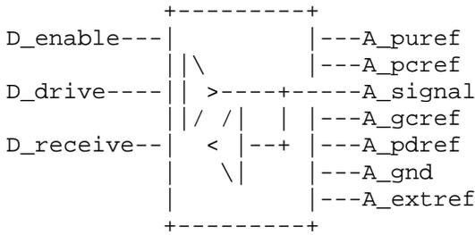
Figure 2: Port names for I/O buffer
