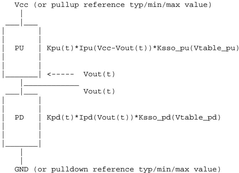
The  $V_{table\_pd}$  and  $V_{table\_pu}$  values may change at each time step. The  $K_{sso\_pd}(V_{table\_pd})$  and  $K_{sso\_pu}(V_{table\_pu})$  values are derived from the dynamic reference voltage variation and [ISSO PD] and [ISSO PU] table entries according to the formulas below:
