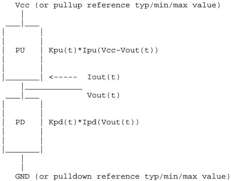
When the supplies are modulated during simulation, the modulation coefficients  $K_{sso\_pu}(V_{table\_pu})$  and  $K_{sso\_pd}(V_{table\_pd})$  modify the equations as shown:
