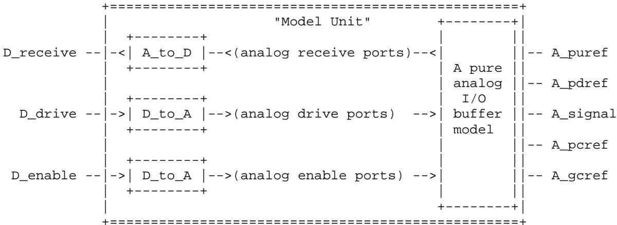
Model Unit consists of SPICE, VHDL-A(MS), Verilog-A(MS) code plus
