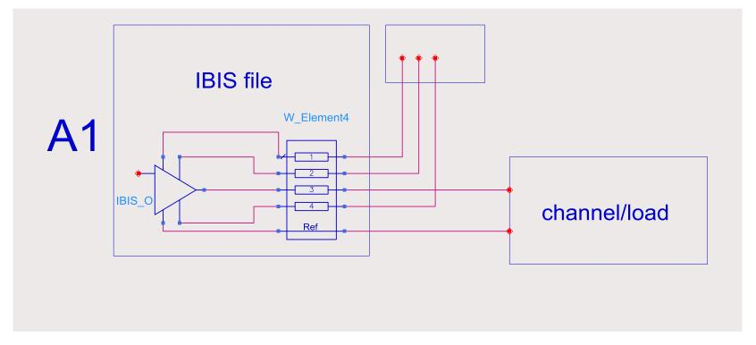
Case A is a superset. The rails sharing the same [xxx Reference] values collapse to common rails.
