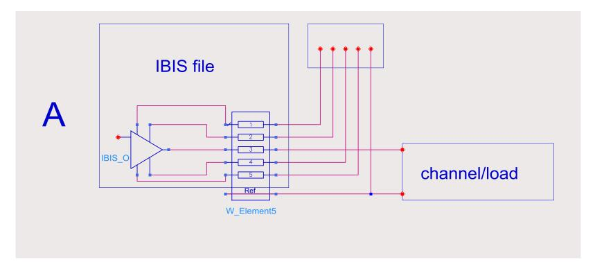
The Ref rail represented 0.0 V, though in simulation it did not have to be connected to node 0 – "GND" instead of the ground symbol was better.
