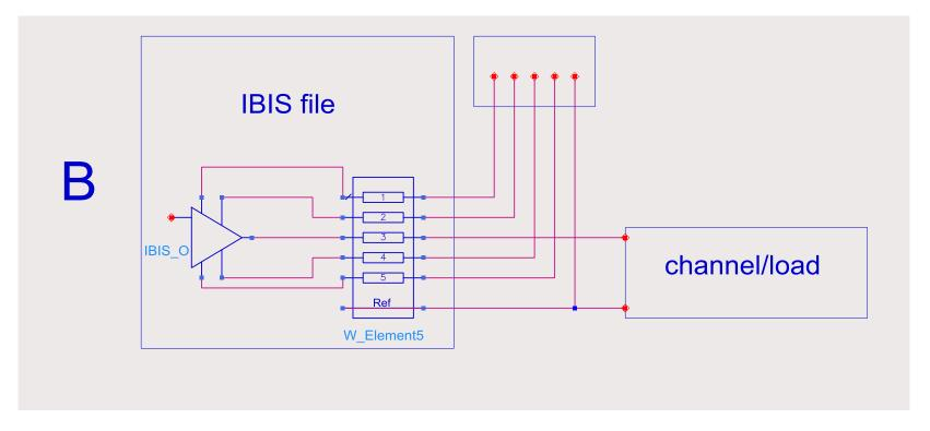
Here, the reference node is one of the pins of the component. The previously proposed [Pin Reference] keyword could facilitate this and provide means for the model makers to identify it (optionally).
