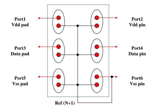
The 6-port (.s6p) S-parameter model of the 6-terminal package model "This reference node could be connected to a POWER or GND pin of the component..."
