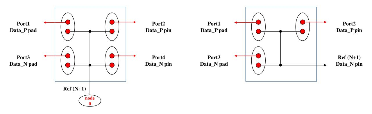
Define the N+1 terminal as an "extra" connection to node 0? Force model makers to generate "NumberOfTerminals-1 port" S-parameter models?
