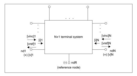
**Figure 1: Terminal Node Notation**
