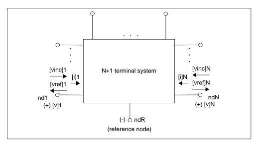
Figure 27 Terminal Node Notation
