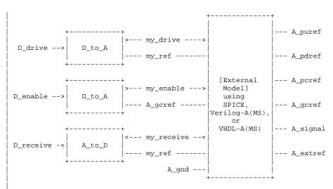
Figure 7: Example of an [External Model] I/O buffer using SPICE, Verilog-A(MS) or VHDL-A(MS)
