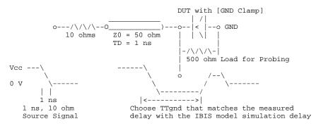
Example of TTgnd Extraction Setup
