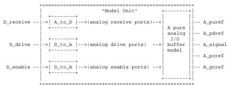
Model Unit consists of SPICE, VHDL-A(MS), Verilog-A(MS) code plus  $A_{to_D}$  and  $D_{TO_A}$  converters (references for  $D_{to}A$  and  $A_{to}D$  converters not shown)
