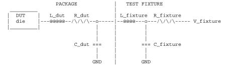
NOTE: The use of L\_dut, R\_dut, and C\_dut is strongly discouraged in developing waveform data from simulation models. Some simulators may ignore these parameters because they may introduce numerical time constant artifacts.
