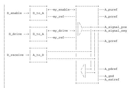
Figure 11: Example SPICE, Verilog-A(MS) or VHDL-A(MS) implementation of a true differential buffer
