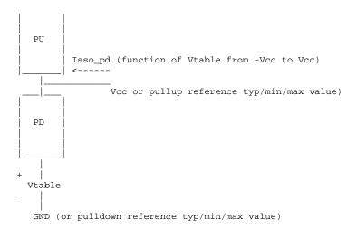
The effective current table for the Isso\_pu current is extracted by the following process. The buffer is set to "logic one". A Vtable voltage source is inserted between the [Pullup Reference] node and the buffer as shown below. This Vtable voltage is swept form -Vcc (typical) to +Vcc (typical) and is relative to the [Pullup Reference] typ/min/max values for the corresponding columns. The output is connected to the Vcc (typical) value as shown below.
