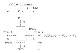
Either of the FETs could be removed (or have zero current contribution). Thus this model covers all four conditions, off, single NMOS, single PMOS and parallel NMOS/PMOS.
