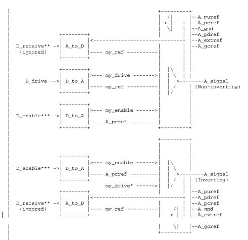
Figure 8: Example SPICE, Verilog-A(MS) or VHDL-A(MS) implementation
