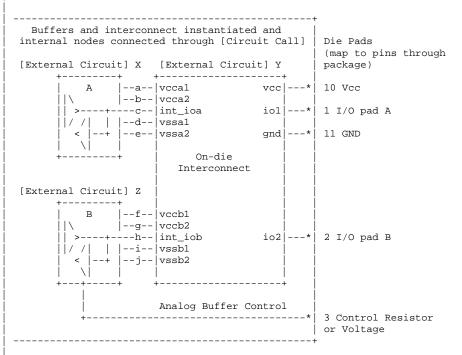
Figure 4: Example showing [External Circuit] ports
