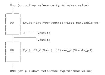
The Vtable\_pd and Vtable\_pu values may change at each time step. The Ksso\_pd(Vtable\_pd) and Ksso\_pu(Vtable\_pu) values are derived from the dynamic reference voltage variation and [ISSO PD] and [ISSO PU] table entries according to the formulas below:
