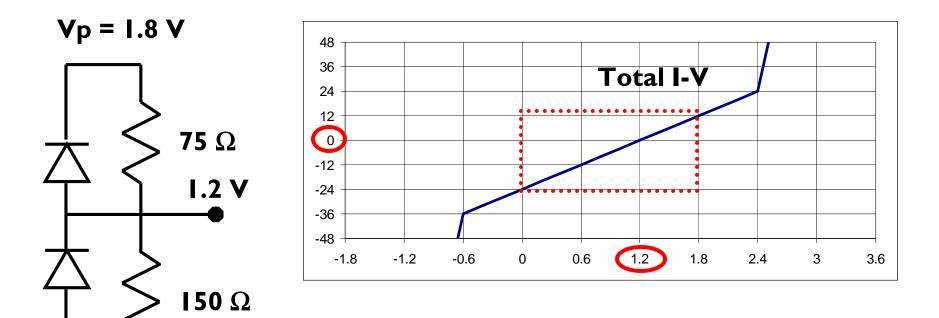
50  $\Omega$  Total I-V curve with 0.6 V "stick" diodes anchored to each rail
